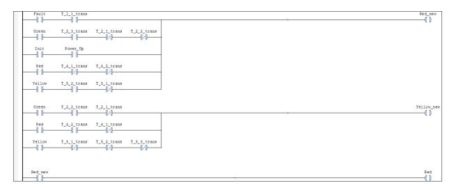
You can map elements of the original Stateflow chart to these coils and contacts. For instance, the coil Red\_new corresponds to the update of the state Red in the Stateflow chart. For the coil to receive power, one of the following must be true:
