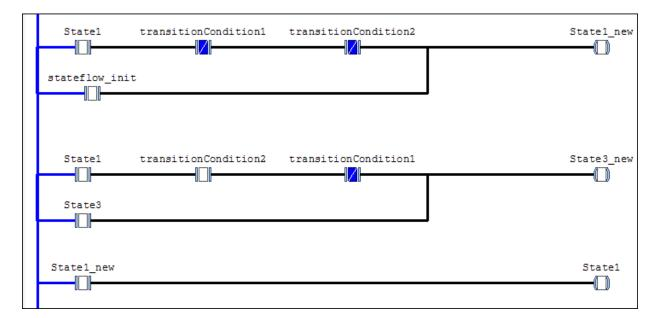
In the preceding ladder diagram, each rung of the ladder ends in a coil. The coil corresponds to a state of the original chart. The contacts before the coil determine if the coil receives power. You can compare the ladder diagram visually with the Stateflow chart. For instance, the coil State1\_new receives power in one of these two cases:
